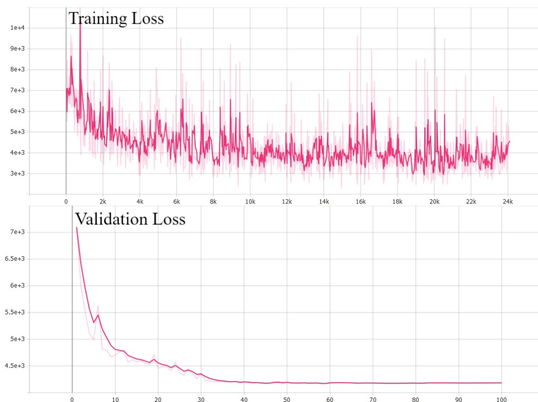
Figure 12. Loss Plot with Learning Rate Decay. The vertical axis is the weighted Adaptive Wing loss. For the training loss, the horizontal axis is the number of iterations. For the validation loss, the horizontal axis is the number of epochs.
