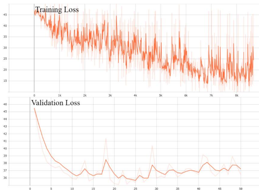
Figure 6. Loss Plot after Hyperparameter Tuning. The y -axis is the MSE loss. For the training loss, the x -axis is the number of iterations. For the validation loss, the x -axis is the number of epochs.
